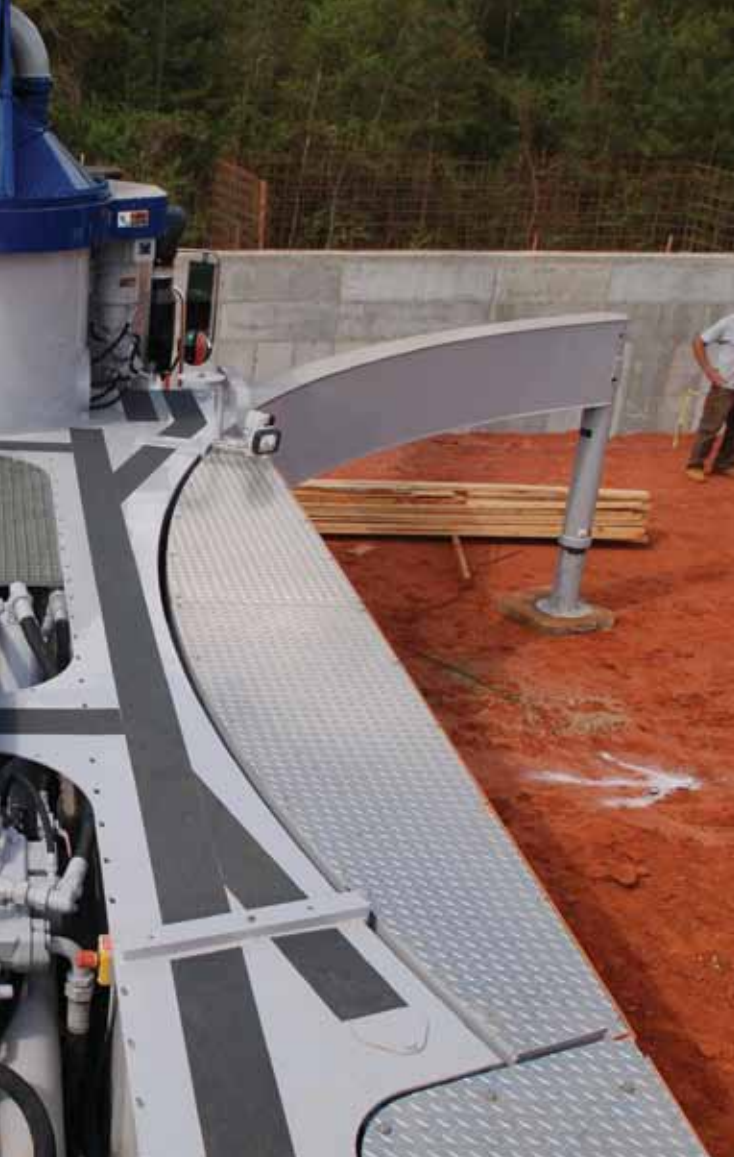
Curved outriggers provide a stable pumping platform with a small footprint.
